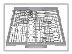
A separate arrangement of the cutlery makes collection easier after washing and improves washing and drying performance. The geometry of the rack makes it possible to place such small items as coffee cups in the area in the middle.
